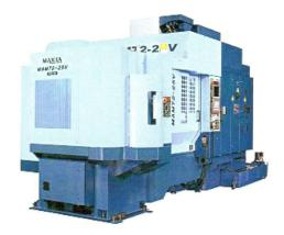
(ONE) FIVE-AXIS MITSUBISHI HORIZONTAL CNC FLEXIBLE MACHINING CENTER Model MH50C with 60 Tools, Fanuc Model 11M Control, Two Pallet Shuttle System with 20" x 20" Table, 28" x 25" x 25" Envelope, Inductosyn Scales, 360,000 Position (0.001 Degree Resolution) Rotary Table, 4000 RPM, 15 H.P., and 1760 lb. maximum piece weight, and chip conveyor.
