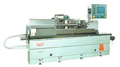
(ONE) OKAMOTO LINEAR B SERIES 612 With Heidenhain 3 Axis, P.G. Optidress, Grind-Rite Centerless, Model 15-000, Coolant System with Splash, adapter bracket and special 8" wheel guard.
